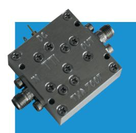
TTI-LNA-X-SKA5 is a warm broadband low noise amplifier highly integrated in a compact package.
